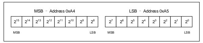
Figure 16. CYCLECNT Register Format
