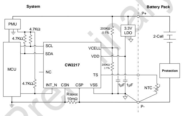
Figure 27. Typical Application for 2-Cell System Side
