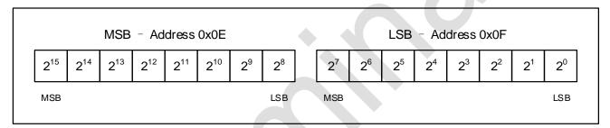
Figure 13. CURRENT Register Format
