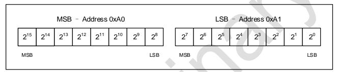
Figure 14. T\_HOST Register Format
