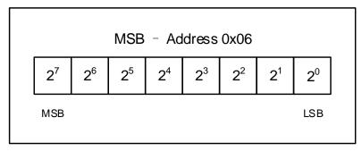
Figure 7. TEMP Register Format
