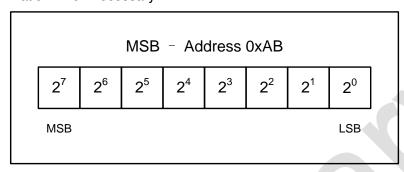
Figure 19. FW\_VERSION Register Format
