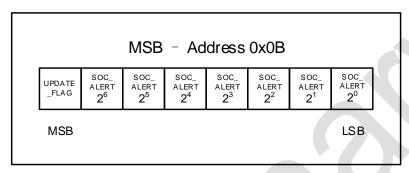
Figure 10. SOC ALERT Register Format
