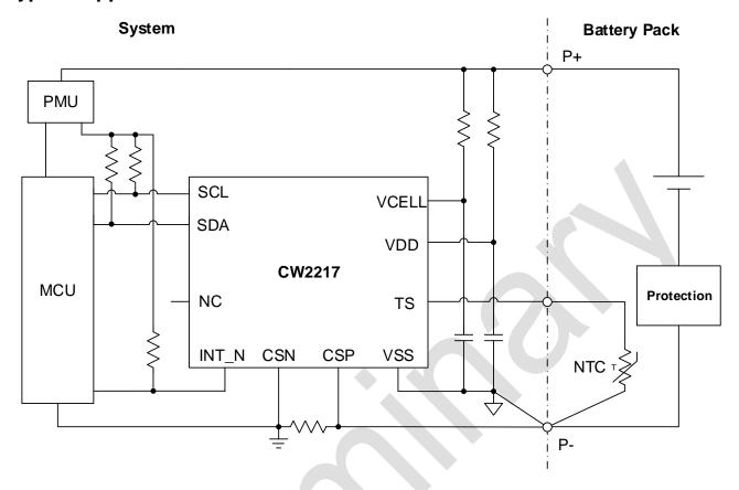
Figure 1. Typical Application for Single Cell
