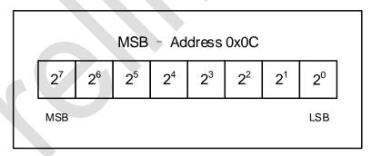
Figure 11. TEMP\_MAX Register Format
