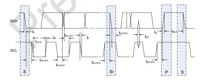
Figure 2. I<sup>2</sup>C Timing Diagram
