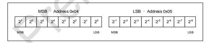
Figure 6. SOC Register Format
