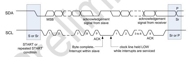
Figure 22. Data Transfer on the I2C Bus
