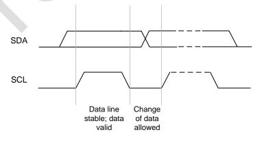
Figure 20. Bit Transfer on the I2C Bus
