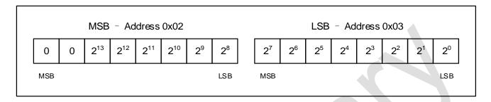
Figure 5. VCELL Register Format
